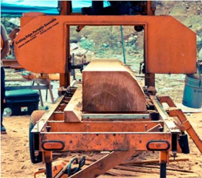
Above and Side: The portable mill. Logs are placed directly onto the mill, and can be cut into the specifications needed.
