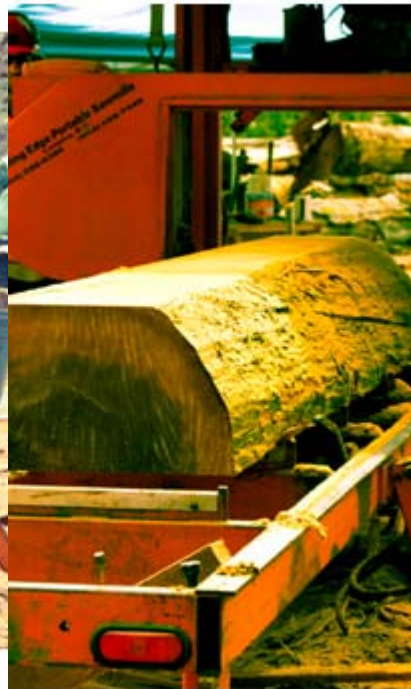
Above and Side: The portable mill. Logs are placed directly onto the mill, and can be cut into the specifications needed.
